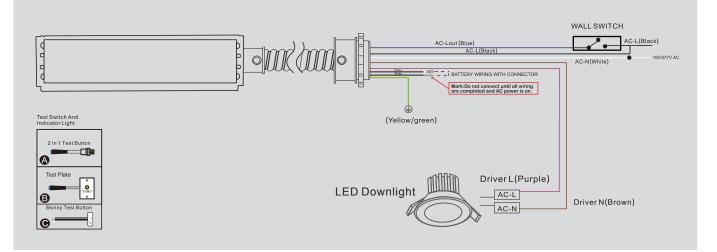
Emergency Driver can be used with either a switched or unswitched or emergency only fixture. If a switched fixture is used, an unswitched hot lead must be connected to the emergency driver.
