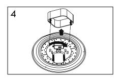
4. Securely mount the fixture plate to the junction box firmly.
