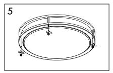
5. Place Diffuser and tighten screws clockwise to complete the installation. Restore power to the electrical box. Turn the light switch on to activate the fixture.
