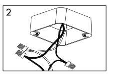
2. Open the junction box. Junction box contains three wires: hot (black), neutral (white) and bare ground. Connect the two hot wires together with wiring nuts (one from the light switch cable and the other from the recessed housing). Repeat the step with the two neutral wires. Close the junction box to complete the wiring.
