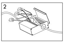
2. Open the junction box. Remove the knockouts for wiring. Junction box contains three wires: black (hot), white (neutral) and bare ground. Insert the white (neutral) supply wire into quick wiring connector with the preassembled white fixture wire. Repeat the step with the two hot wires and ground wires. Close the junction box to complete the wiring.
