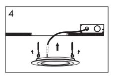
4. Push the easy mount clips up and insert the downlight into the ceiling, release clips to mount the downlight on the ceiling.
