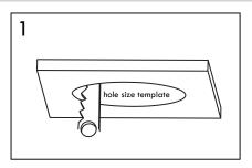
1. Use the hole size template in the packaging to cut a hole on the ceiling for installation.
