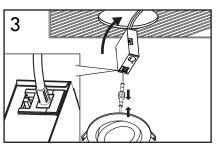
3. Connect downlight to junction box. Select your favorite color temperature by using the 5CCT switch on the junction box. Place junction box into the ceiling.
