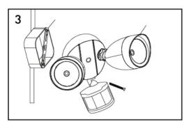
3. Align mounting holes of lamp body(A) to the crossbar(D), secure with the provided plate screw(E) and complete the installation.
