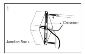
1. Attach the crossbar (D) to the junction box (not included) with the screws (B).
