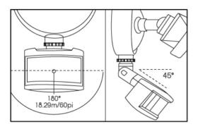
Note: Do not aim the sensor at the water, plants that will move in the wind, rain and traffic etc. as those will trigger the sensor. Make sure the joint screws in the sensor arm are tightened.
