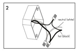
2. Connect the fixture to 120Vac 60Hz circuits. Junction box contains three wires: hot (black), neutral (white) and bare ground. Connect the two hot wires (one from the light switch cable and the other from the recessed housing) together with wire nut (C). Repeat the step with the two neutral wires and ground wires. Close the junction box to complete the wiring.
