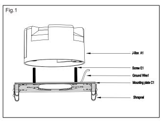
1. Secure the mounting plate (C1) to the junction box (A1) using junction box screws(E1). The side of the mounting plate marked "GND" (C1) must face out.
