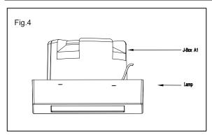
4. Snap the lamp into the housing firmly. Make sure the light is secured to complete the installation. (Fig.4)
