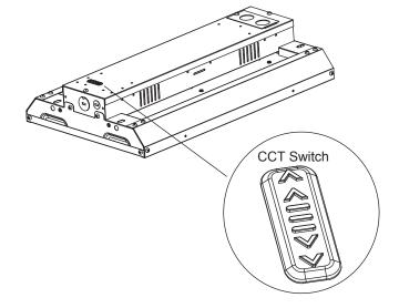
The end users may adjust the color temperature by the DIP switch buttons integrated into the driver. The DIP switch is accommodated with 2 options (left and right), corresponding to 2 color temperatures, which can perform the desired color temperatures.
