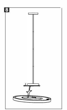
8. Connect supply wires from themounting bracket to the supplywires of the luminaire.
