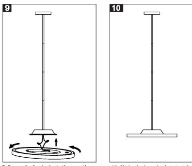
9. Secure the luminaire to themounting bracket by rotating theluminaire clockwise.
