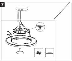
7. Connect LN wires from the luminaire to LN wiresfrom mounting bracket, then secure the anti-releasesteel wire on the mounting bracket and rotate theluminaire in the direction as Figure 7 to lock.
