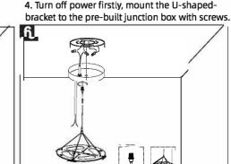
5. Connect the LN wires from the pendant to theexternal input LN wires. and U-shaped bracketground wire to the external input ground wire.
