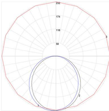
Maximum Candela = 232.14 Located At Horizontal Angle = 157.5, Vertical Angle = 4
