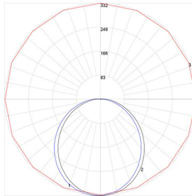
Maximum Candela = 331.95 Located At Horizontal Angle = 112.5, Vertical Angle = 3
