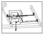
2.Repeat step 1, put the construction can and on another side fix the brackets with nails.
