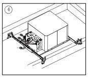
4. Knock out the knock hole and assemble the flexible metal conduit. Open the junction box, and connect the house wire accurately according to the instruction.
