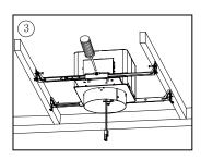
3. Move the constructioncan to the proper location and screw it.
