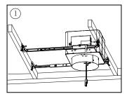
1.Put the construction can on one side and fix the brackets with nails.
